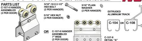
SPECIFICATIONS: -LOAD CAPACITY: C-107-4 HANGERS: 350 LBS PER DOOR C-107-8 HANGERS: 500 LBS PER DOOR
